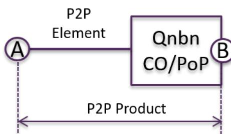
In this structure, a Customer location is connected to a Qnbn CO or Point of Presence (PoP).
